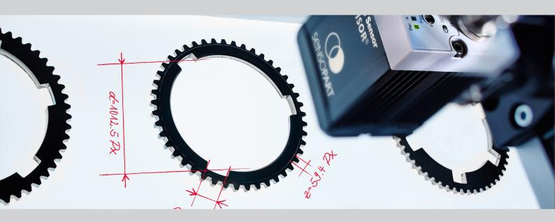
Component position and distance values are generally required in metric units, such as millimeters or inches, rather than in pixels. Thanks to the VISOR® calibration function, vision sensor coordinates can now effortlessly be converted into real-world engineering units: place the calibration plate into the sensor's field of view, a single mouse click in the configuration program – and it's done!
