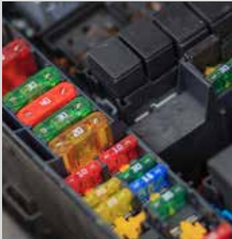
Inspection of car fuses – color and material
