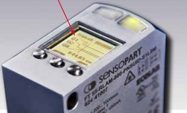
Easy-to-read LCD display simplifies setup
