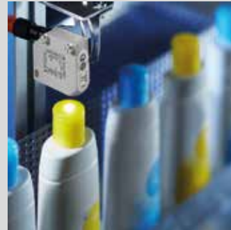
Detection of colored bottle lids A white light FT 50-C color sensor checks the color to detect whether the correct bottle lids are used.
