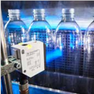
Inspecting presence of transparent bottles The FT 55 BlueLight sensor is used in a bottling plant to check whether bottles are present and correctly positioned.
