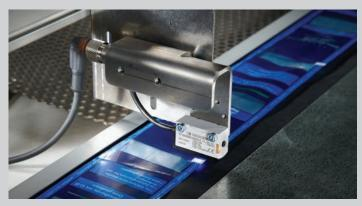
**Out with the old, in with the new:** The contrast sensors from the F 25 series are assembly and connection compatible with the conventional standard housing (image on the left). The fastening bores are aligned in the same distance from each other. The integrated cable with a M12-connector fits to the corresponding mating connector.
