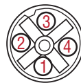
Female, 4-pin (M12-D) integral connector pin-out as viewed from the end of the sensor
