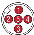
Male, 5-pin (D54) integral connector pin-out as viewed from the end of the sensor
