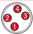
Input voltage, male, 4-pin (D54) integral connector pin-out as viewed from the end of the sensor
