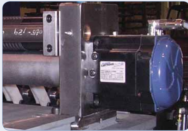
Same machine with a Cartridge DDR motor installed. Here, the shaft of the driven roll is extended into the Cartridge DDR motor and the motor applies torque directly to the driven roll.
