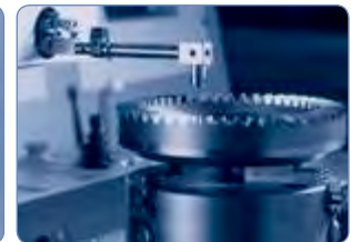
Computerized mapping of gear tooth profile
