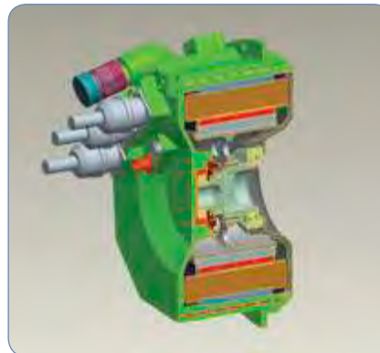
200 kW electric starter/generator
