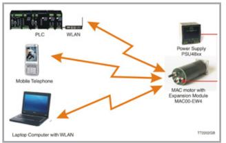
Examples of communication possibilities with the WLAN Expansion module. Note: Only one of the possibilities can communicate at a time.
