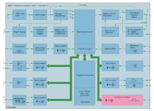
The diagram above shows schematically the internal structure of the AMC AC Servo Controllers. All inputs and outputs are available via a multi-connector (DIN41612 ver. C) on the rear panel. A connector board CON13 enables connection via screw terminals (Phoenix plug). The RS232/485 interface is available via a 9-pole SUB-9 connector on the Controller's front panel. The front panel is also equipped with LEDs that indicate Controller status.
