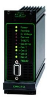
DMC10 is a compact, programmable DC servo motor controller.
