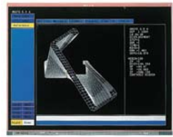
Deformation of a competitor's base structure under the same amount of force.
