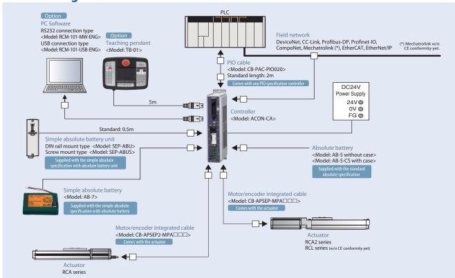
■ If the RCA/RCA2 actuator is operated with the ACON-CA, specify "A5" as the applicable controller for the RCA/RCA2.
