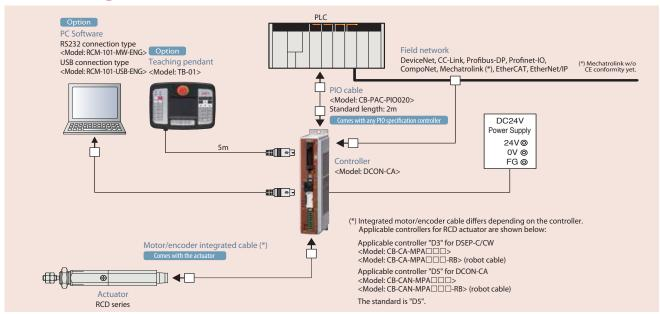
■ When the actuator RCD is moved by DCON-CA, the call-out for the applicable controller of RCD is "D5".
