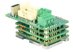
The **FXM060-5-EM** is an Extended Environment single-axis servo drive and integration board assembly for a FXE060-5-EM FlexPro<sup>™</sup> series servo drive with IMPACT<sup>™</sup> architecture. Connections to the controller, motor, power, and feedback are simplified through the standard connectors featured on the board.
