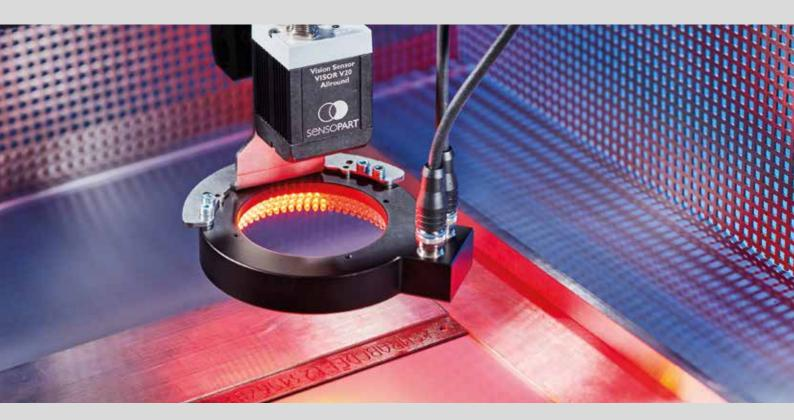
Raised or recessed object details – such as embossed digits and characters on a credit card – are difficult to detect with standard image processing methods. Even use of lateral lighting generally results in poorly identifiable contours due to overexposure and shadows. The solution comes in the shape of SensoPart's VISOR® vision sensor series with the new multishot function.
