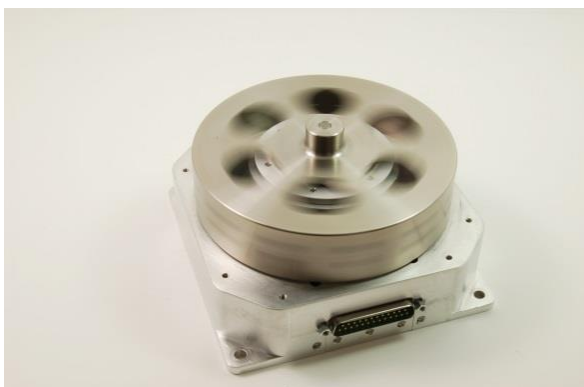
maxon motors drive the reaction wheels that control the inclination of the satellite. © Clyde Space
