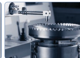
Computerized mapping of gear tooth profile
