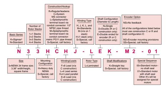
The example model number above indicates a N series standard NEMA 34 frame motor with a three stack rotor. This motor is equipped with a heavy duty front end bell and shaft, and a sealed system rear end bell with MS connectors. It also has a bipolar parallel connection, a J winding, a straight keyway, encoder mounting options and a shaft seal.
