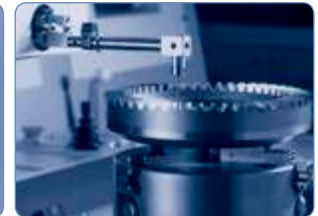
Computerized mapping of gear tooth profile
