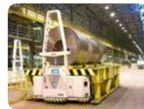
World's first driverless vehicle with 16 controlled wheels, Posco Steel, South Korea, 2009
