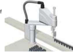
Example: Palletizing of loads using a SCARA robot
