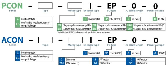
\* If a RCA-RA3  $\square$  /RGS3  $\square$  /RGD3  $\square$  or RCA2-SA4  $\square$  /TA5  $\square$  is to be connected, specify 20S for the motor type.
