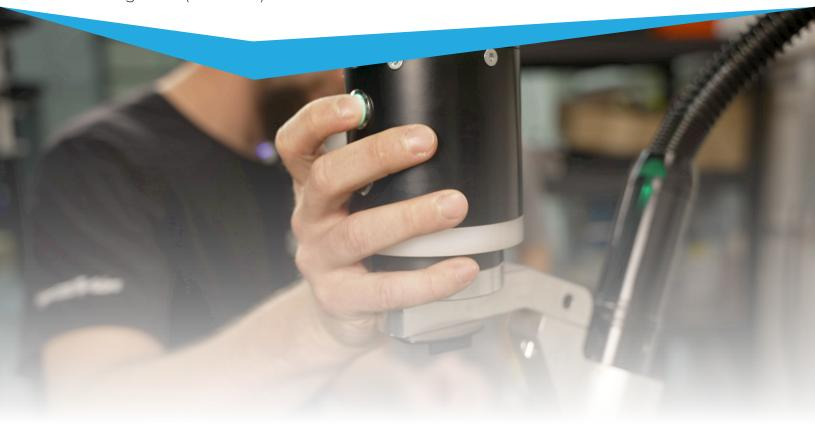
Hirebotics did also develop their Smart Puck device that is installed on the robot flange. Its use is to teach your Cobot Welder to weld anything without touching the teach pendant. You can then create weld waypoints with two buttons; use the green-lighted button to move the arm in freedrive and the blue-lighted button to record the position. Easy peasy!
