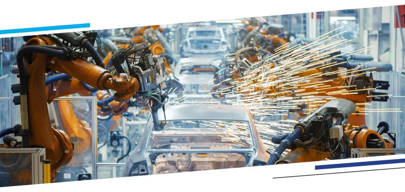
They are big and bulky and are made for high-volume production. They also require complex programming. These robots can be more expensive with their rigid installation and jigs placed in a robotic welding cell. They are not so much a fit for the low volume, high mix environments of most small and flexible welding operations.
