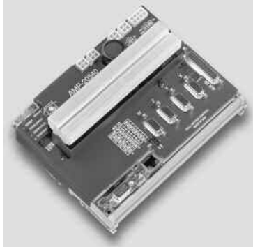
AMP-20540 Interconnect with 4-axis 500 W servo drives
