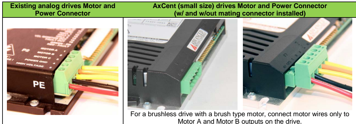
Figure 6 Motor and Power Connector
